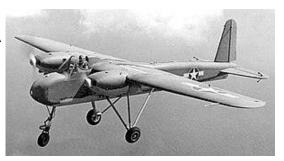
When manned, the TDN-1 had a crew of one with a wingspan of 48 feet and was 37 feet long. Power was provided by two Lycoming six-cylinder 220 hp engines. Cruise speed was 145 mph and it carried one 2000 pound bomb or one aerial torpedo. The first flight was on November 15, 1942. **B**etween 104 and 114 were built.
