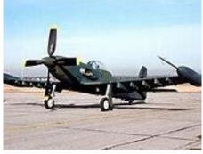
In the 1970's, Cavalier Aircraft built a Light Air-Support Reconnaissance Aircraft (LARA) "Mustang" which was a turbo prop powered engine called the Enforcer. They were later built by Piper as they could mass produce them.
