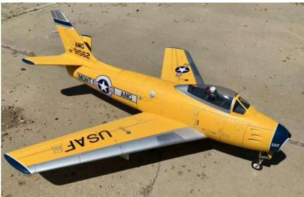
Adam Kremers' Freewing F-86 with 80mm fan. It flies on 6S 4000-4400mah packs. It was modelled after a National Guard target towing aircraft, thus the yellow paint scheme.
