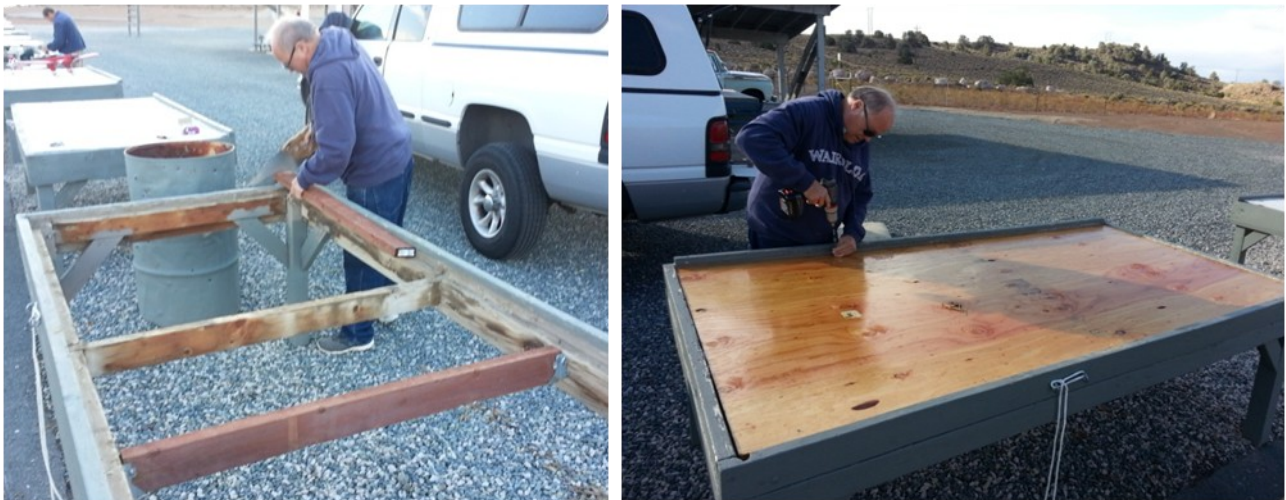
Club President Dan Etcheto working on replacing the rotted table tops with weather-proofed plywood
