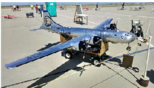
This B-29 is covered with aluminum foil tape used on a/c and heating ducting.
