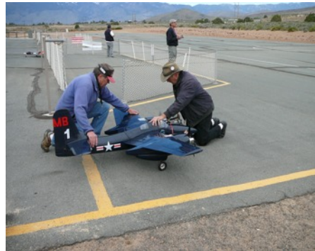
Our first "Pilots Choice Award" went to Ray Brindos for his fantastic Grumman F7F Tiger Cat . This plane is fast, fast, fast. Power is from two four stroke YS 1.70 engines. The kit is from K&P with a wingspan of 82 inches.. Bob Heitkamp helped Ray in the pits and flew the plane as well.. Ray also had a huge Corsair with 85"
