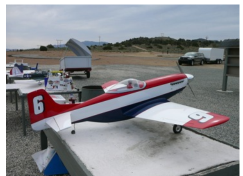
Jim Kelso walks out his 85 inch P-51. Jim builds these models for unlimited Warbird racing. This is powered by an Evolution 58 gas engine.
