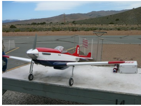
Jim Kelso walks out his 85 inch P-51. Jim builds these models for unlimited Warbird racing. This is powered by an Evolution 58 gas engine.
