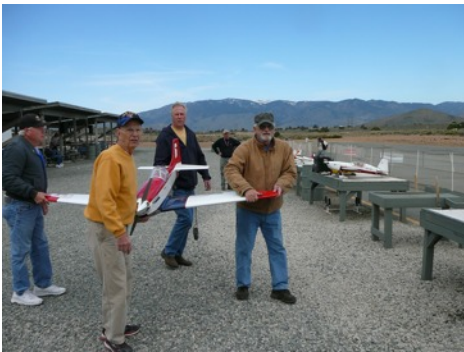
Jim Kelso walks out his 85 inch P-51. Jim builds these models for unlimited Warbird racing. This is powered by an Evolution 58 gas engine.
