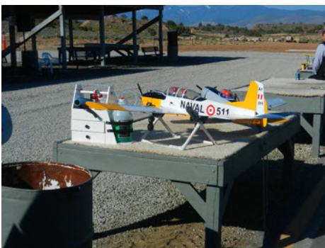
David Belcher's World Models T-34 with the stock racing gear. OS 46 power and 56" wingspan
