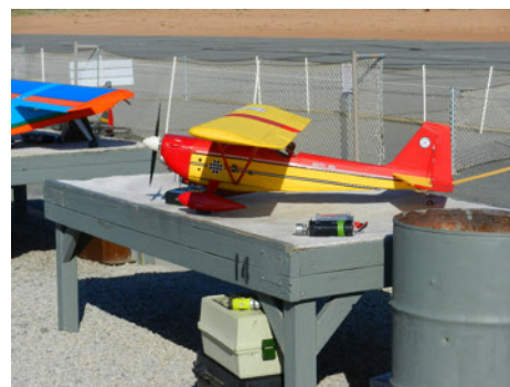
Bob Jones' Citabria Pro RCG 26cc Gas engine, 80" wingspan weighing in at 12 pounds
