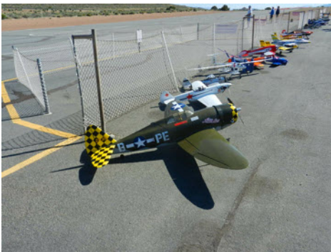
Ray Brindos' P-47, 81" wingspan CRCC 50cc engine for power. Yak-3 sits in the background . Both flew great in the wind.
