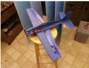
Aerial Combat anyone.... Here are some pics of my foamie Wildcat built for combat and successfully test flown by Les Harris. It has a w.s. of 30" , weighs 8.6 oz ready to fight and is powered by a 1700 kv brushless motor, 10 amp controller and a 1000 mah battery. The foam material is called protection board. It approximately .25 " thick and comes in a sheet 4'x 50' long fan folded.
