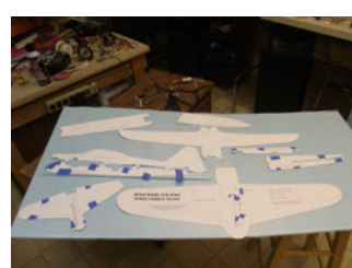
Here are the parts laid out for the Zero to oppose the Wildcat. It will have the same specifications as the Wildcat so their flight characteristics should be similar. Each plane will tow a streamer one inch wide and about 15 feet long. Both planes use two 9 gram servos for ailerons and elevator. Cost per plane should be about *30.00. Stay tuned....and watch your six! -BJ.
