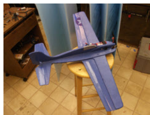
Aerial Combat anyone.... Here are some pics of my foamie Wildcat built for combat and successfully test flown by Les Harris. It has a w.s. of 30" , weighs 8.6 oz ready to fight and is powered by a 1700 kv brushless motor, 10 amp controller and a 1000 mah battery. The foam material is called protection board. It approximately .25 " thick and comes in a sheet 4'x 50' long fan folded.
