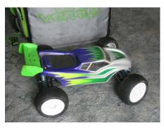
fastest of the 1/8 scale models being raced locally. They can be nitro or electric powered, weigh about 9 lbs and will go about 40 mph in normal race trim. Under ROAR rules a .28 engine is the largest allowed, while most electrics run a 4s 16.8v lipo battery with any appropriate motor.
