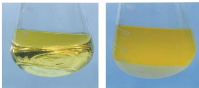
Shown above is an example of phase separation; cloudy suspended water on the right. More next month.....
