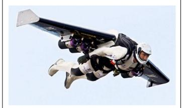
The four German built model aircraft engines he currently uses provide 200lb of thrust each, enough to enable the 110lb foldable carbon wings, and Yves Rossy in his 120lb flying suit, to climb at 200ft a minute.
