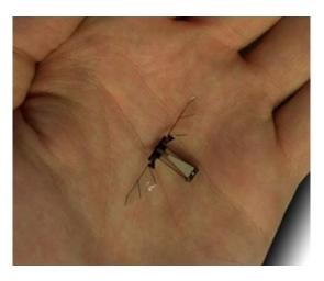
This comes from the fine folks at Harvard School of Engineering and Applied Sciences. Weighing only 60 milligrams, with a wingspan of three centimeters, the tiny robot's movements are modeled on those of a real fly. I am not sure if it is RC controlled or not.
