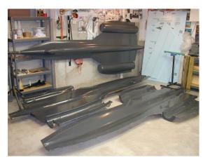
long, and 2 inches short of a 7 foot wingspan. Final dry weight I'm shooting for, is 45 lbs, and is to be powered by 2 AMT Mercuries." Truly amazing workmanship. What you are looking at is the "plug" and the top and bottom "molds."
